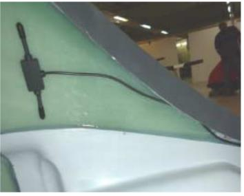
Fix all wires at the left hand cockpit side with cable tie holders and cable ties. You may install some additional cable ties to bundle the wires between the holders.
