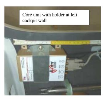
Wire the power supply wires to the distributers (for instruments) in the front instrument tower. Install an on/off switch in the positive wire (to switch off the unit for a reset) and a 0.5A fuse. Install switch and fuse on the front instrument panel. Mark fuse and switch.
