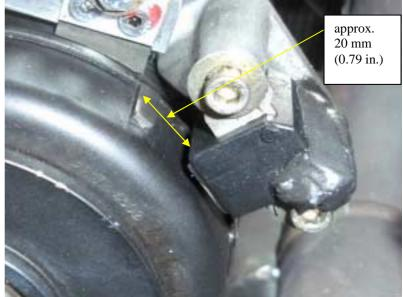
If the drive belt jumped, the problem may be easily corrected with an approx. 30mm wide by 100mm long piece of Mylar tape.
