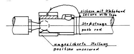
2. For connecting or disconnecting the airbrake control the sleeve must be rotated to make free the opening for the rotule. After engaging the "Hotellier" connectors the sleeve must be rotated 180° to close the opening.
