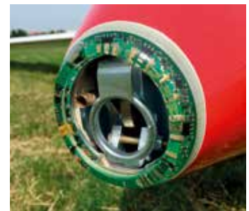
To further enhance safety, a flashlight for the DG-1001 family was designed, which is integrated into the sailplane's nose. The red flashlight significantly adds to crash prevention (photo: DG)
