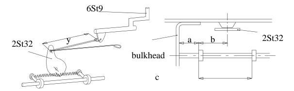
The bungee interconnection between wing flap lever 6 St 9 and trim lever 2 St 32 is to be replaced, when worn or when elongated.
