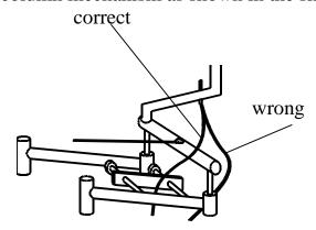
**Warning**: If the cable passes outside the mechanism control column movement can be blocked.
