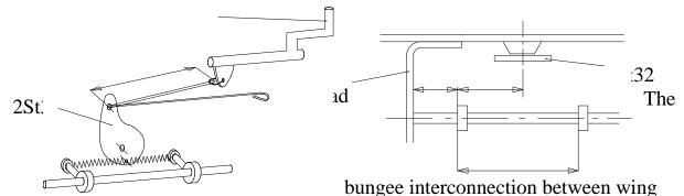
flap lever 6St9 and trim lever 2St32 is to be replaced, when worn or when elongated. The length in unstretched condition y must be 110 mm (4.3 in.). The interconnection consists of 2 mm diameter. bungee wound around 3 times.
