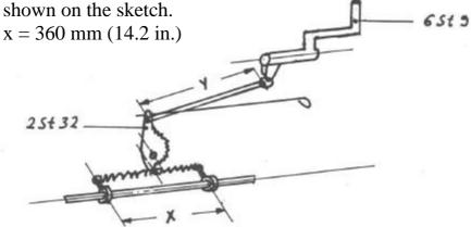
The bungee interconnection between wing flap lever 6 St 9 and trim lever 2 St 32 is to be replaced, when worn or when elongated.
