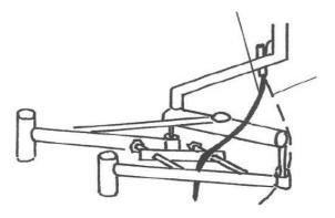
Note: if the cable passes outside the mechanism control column movement could be blocked
