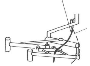
Note: if the cable passes outside the mechanism control column movement could be blocked
