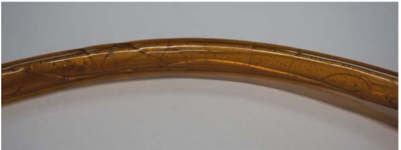
PU hose with crack lines starting at the inside of the hose
