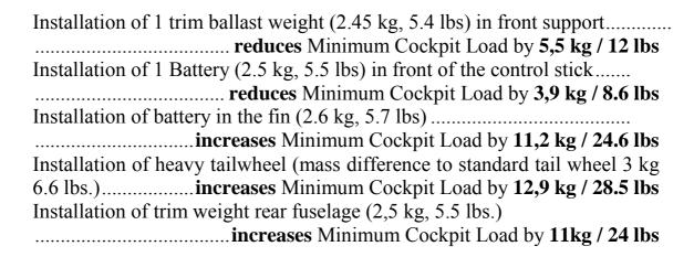
**Warning:** In case of doubt: Mass and Balance must be determined by reweighing the sailplane
