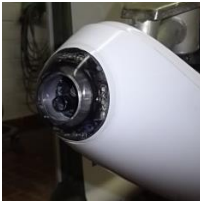
Figure 1, fuselage nose of the DG-single seater with FLASH LIGHT/Safety-flash
