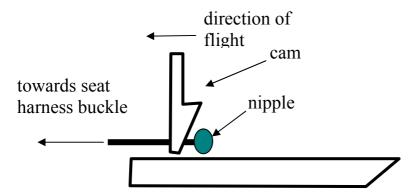
detail of the actuation unit (at the right hand side cockpit wall in front of the main bulkhead)
