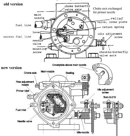
Normal position of the fine adjustment nozzle is fully anticlockwise (open). For high altitude operation the nozzle may be turned in clockwise direction (closed).
