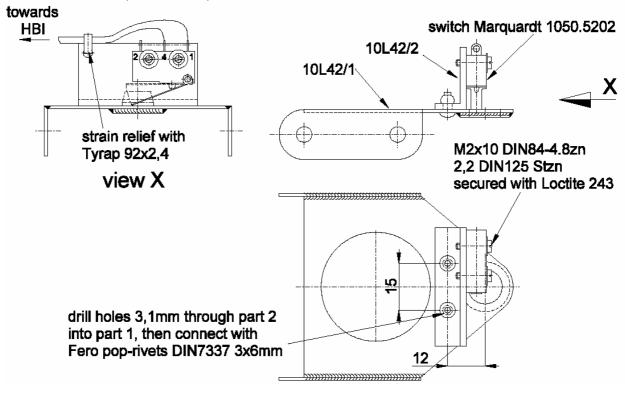
Solder the 2 free wires which come out of the plug of the modified box for the ballast-info to the switch (see sketch).
