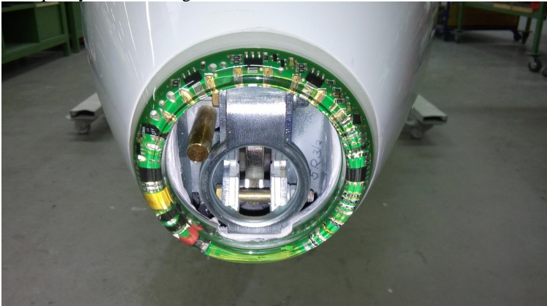
Figure 1, fuselage nose of the DG-1000 with aero tow release and FLASH LIGHT
