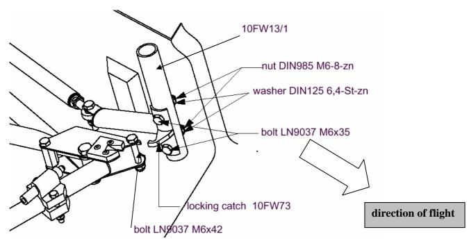
Installation of the locking catch. View LG retracted, locking catch not engaged
