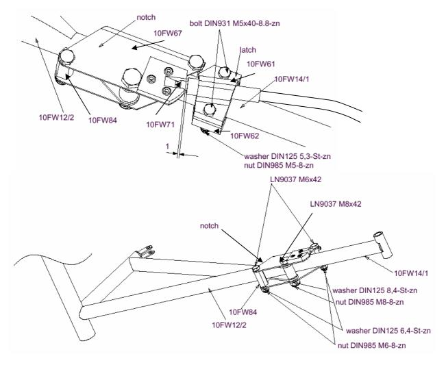
installation of the notch (LG extended) to 10FW12/2
