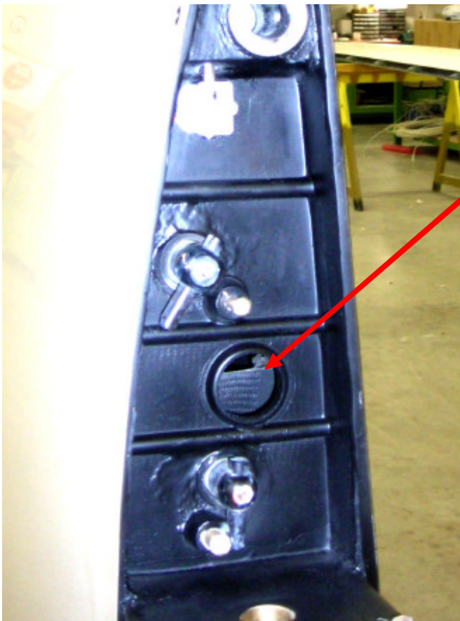
photo 2: root rib with access hole
