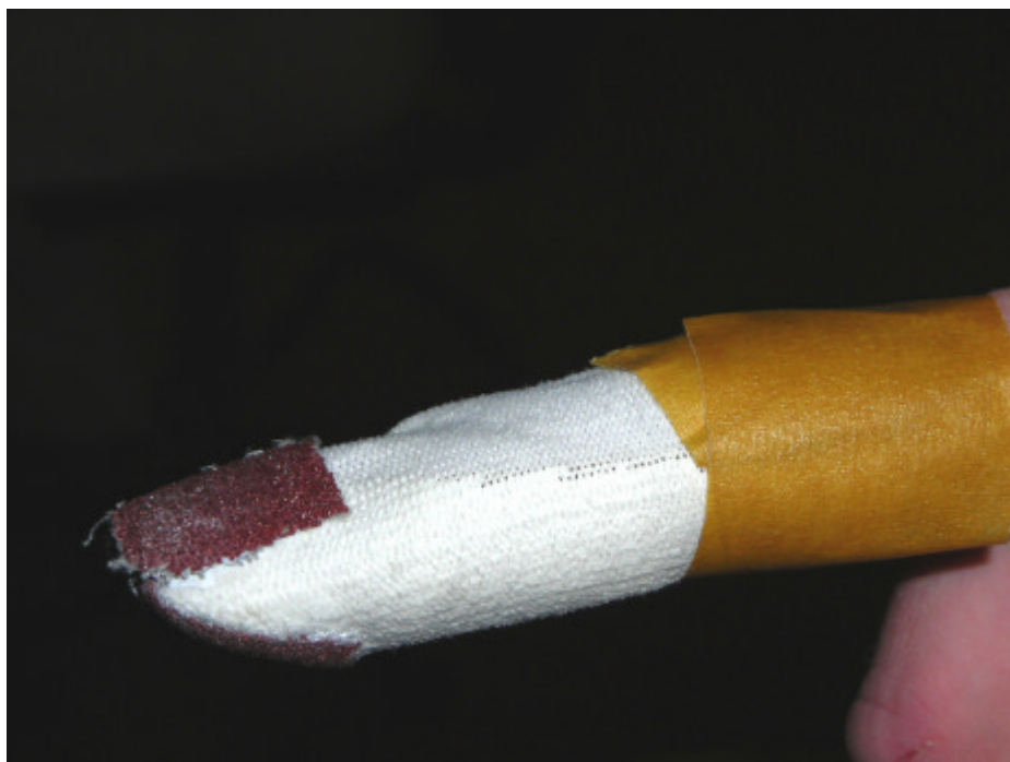
photo 3-4: finger of one time use glove with abrasive paper
