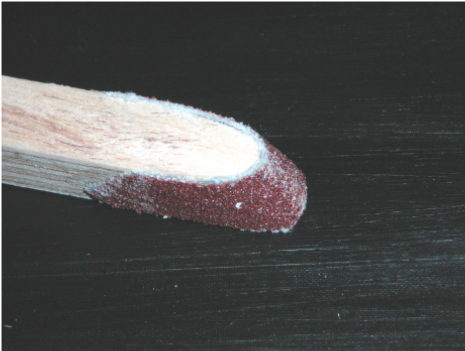
photo 3-2: chamfered and rounded end of the square wooden strip with abrasive paper
