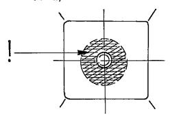
If the washer with 18 mm outside diameter is visible you can reassemble the control lever. Use a new self locking nut M 6 DIN 985.
