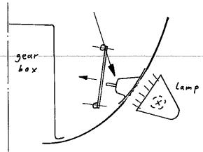
Remove the self locking nut M 6 DIN 985 from the bearing stand and draw off the control lever.
