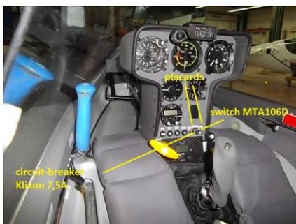
**Picture4:installation of switch and circuit-breaker**
